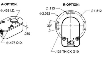
A-Option: Adds a .497" diameter alignment R-Option: Adapter is an 1/8" thick fiberglass shoulder designed to slip into a .500" adapter which is pre-mounted to the base diameter recess in the mounting surface of the encoder. It allows the encoder to rotate +/- 15 degrees.
